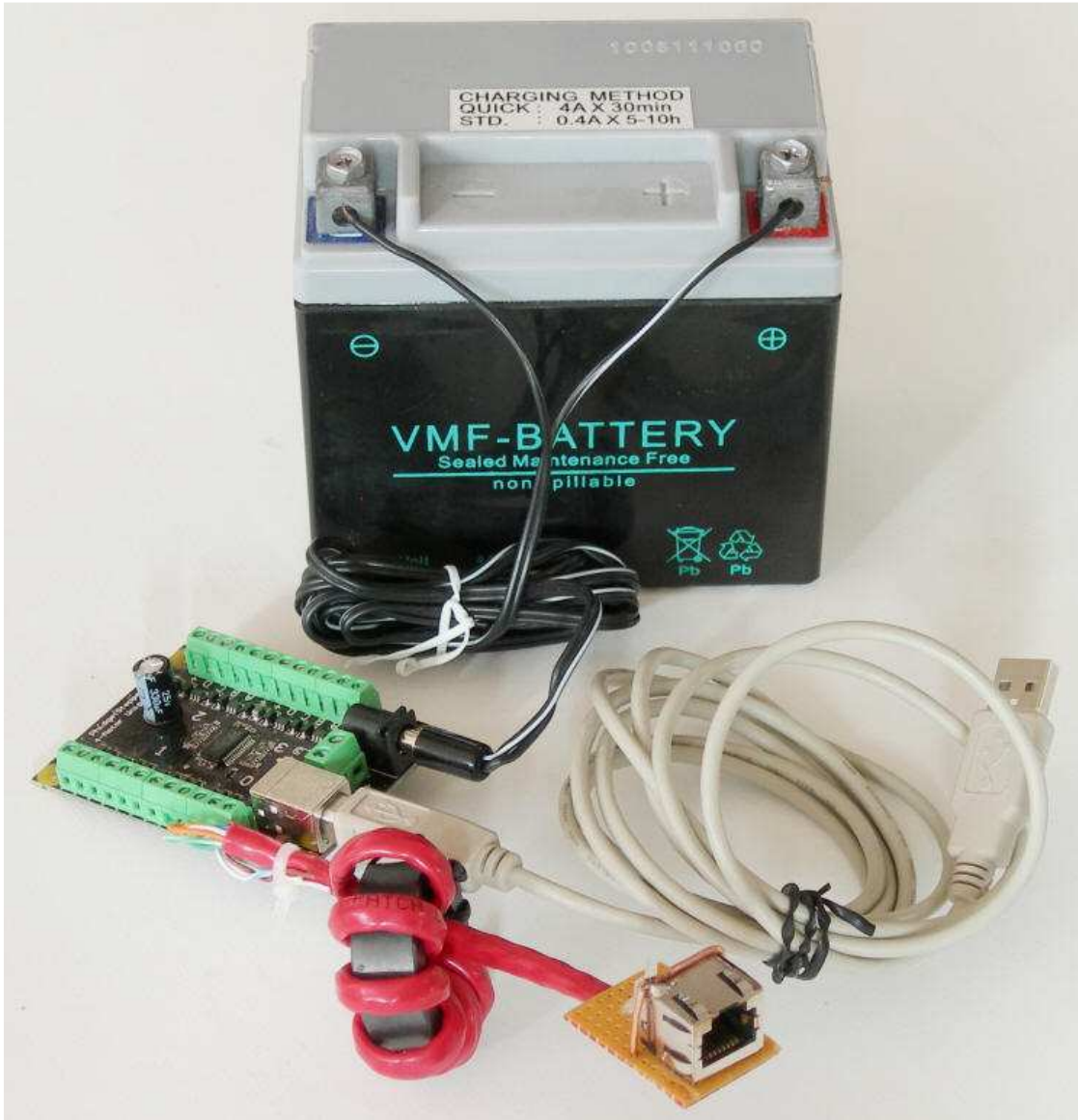
The ferrite choke at the card end of the CAT5 cable to the motor
