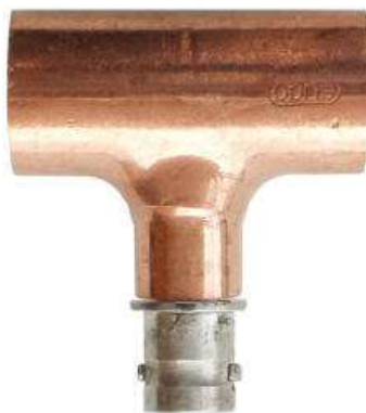
For Gamma Match: BNC chassis connector fits perfectly into 10 mm OD end of a T-piece
