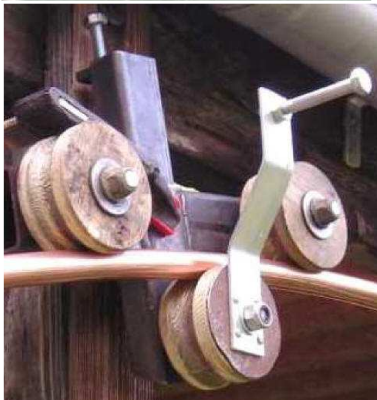
Tube roller made by Twan, PA0KV (photos used with permission)
