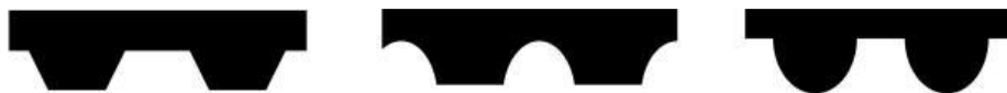
Standard metric belt profiles (left to right: T, AT, HDT) (similar British/Imperial profiles are L, H, XL, MXL)
